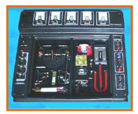
The magnetic set is that part of the Electrolab which deals with magnetic and electromagnetic phenomena. The magnetic set may be purchased separately. Molded plastic compartments with legend ensures that no parts are mislaid at the end of the session.
